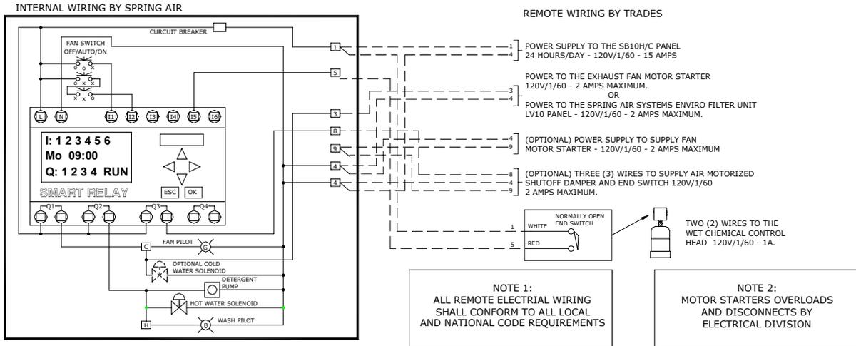
Typical KES wiring to SBA10C water wash panel
