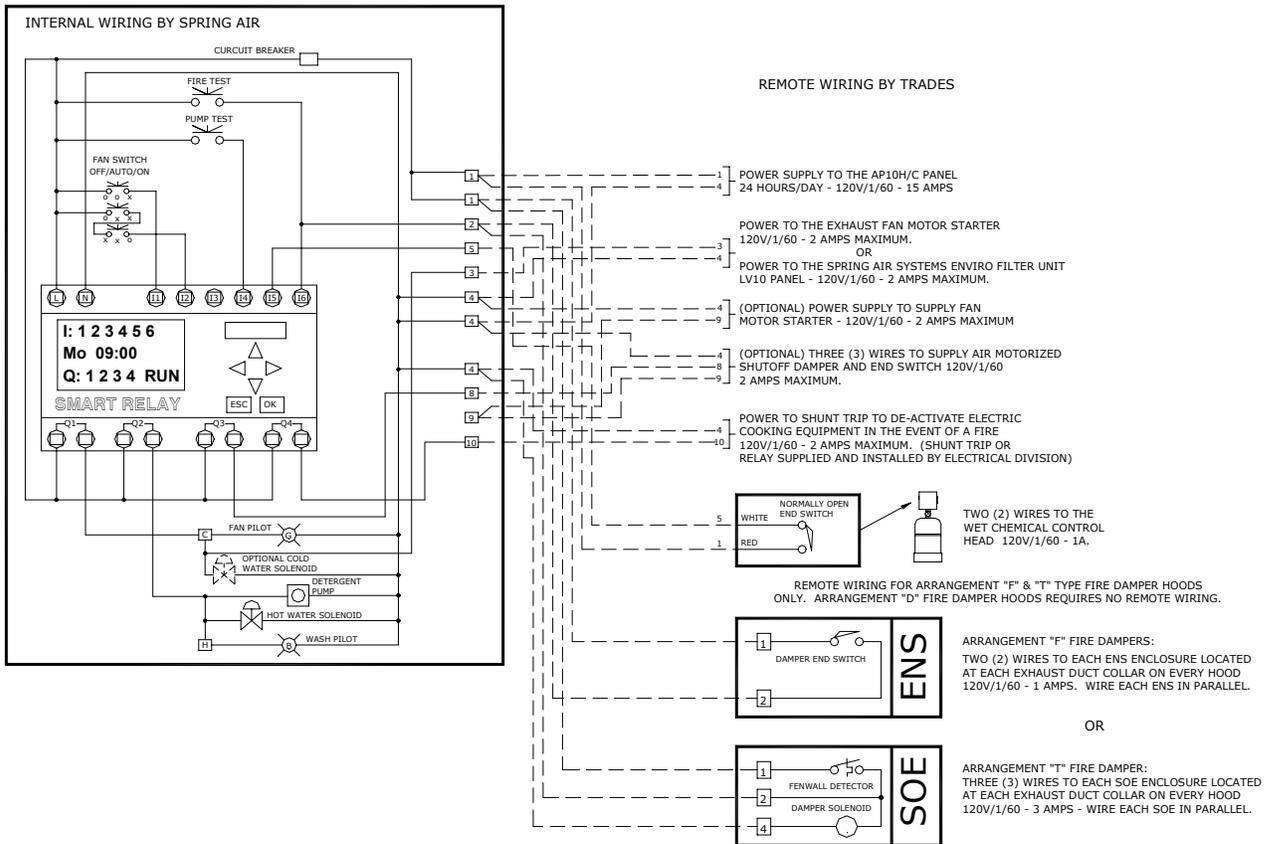
Typical KES wiring to AP10H water wash panel
