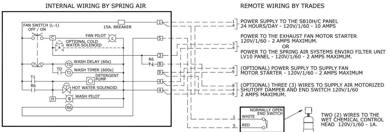
**Typical KES wiring to SB10C water wash panel**
