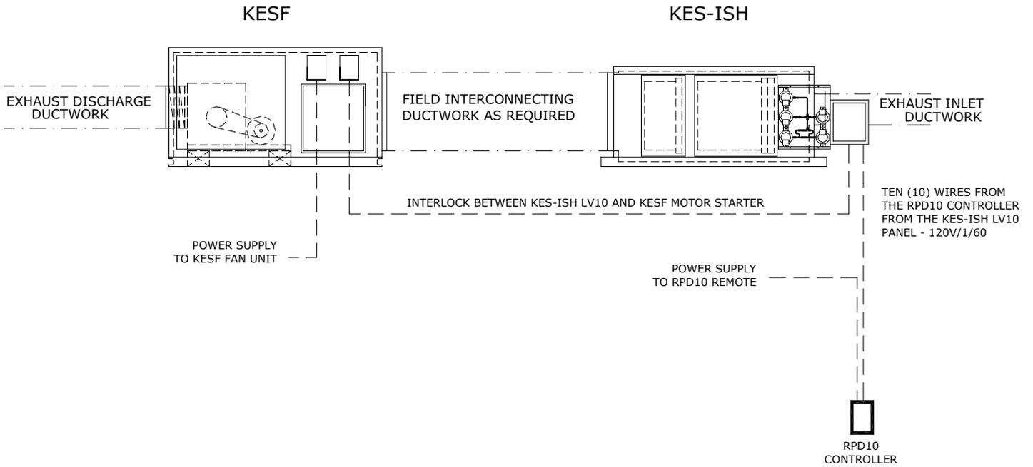
Remote wiring of KES enviro units with Dry Hood
