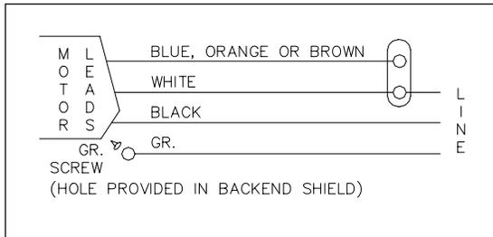
For any permanent split capacitor motor, which has four(4) leads is as follows:
