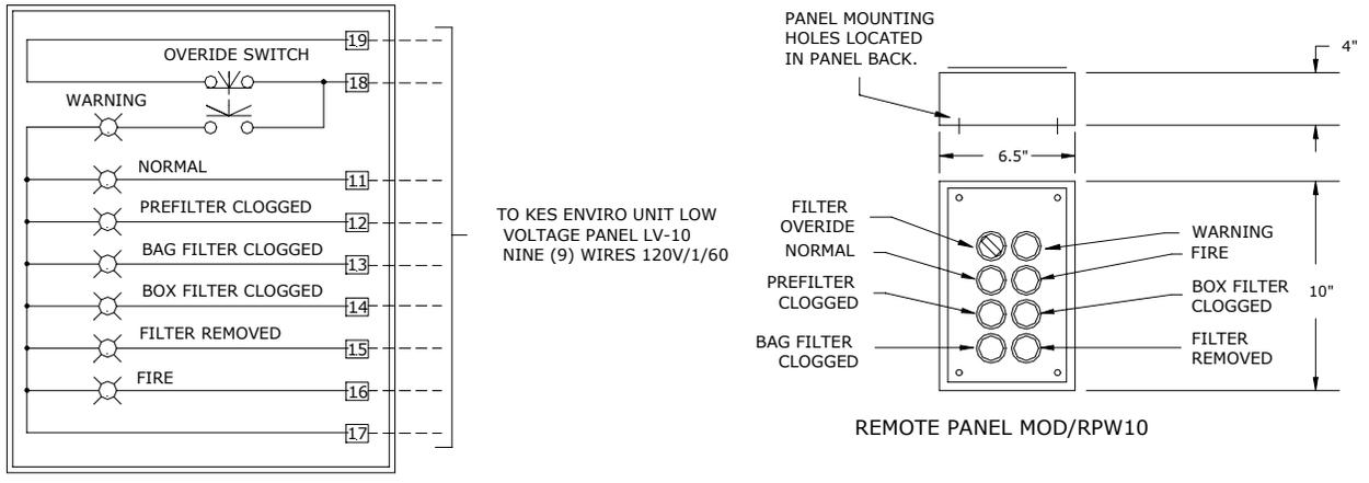
RPW10 internal wiring schematics
