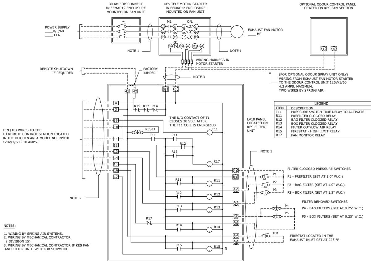
Wiring diagram for LV10 panel with RPD10 and motor starter
