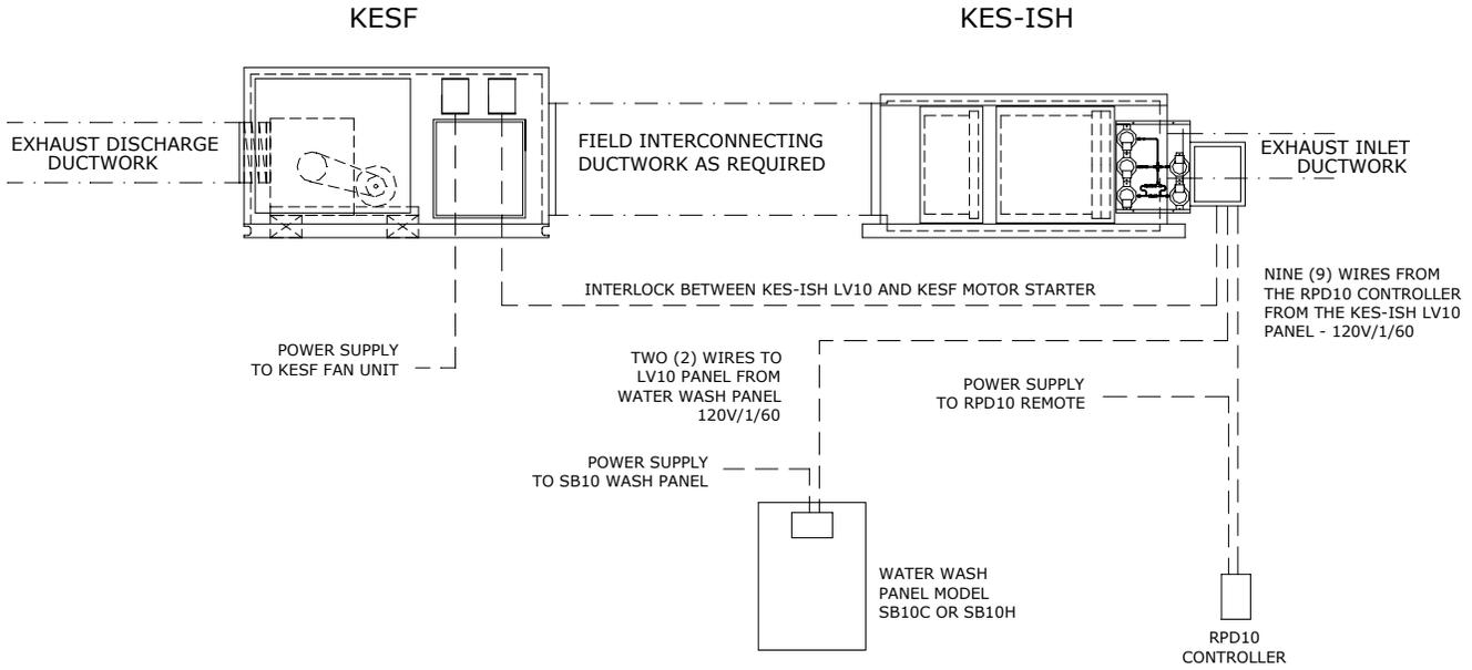
Remote wiring of KES enviro units with Water Wash Hood and Panel
