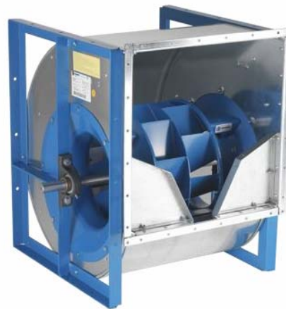
A KESF DWDI fan. Correct rotation for this fan arrangement looking into the end shown above is clockwise Figure 29
