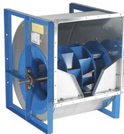
A KESF DWDI fan. Correct rotation for this fan arrangement looking into the end shown above is clockwise Figure 29
